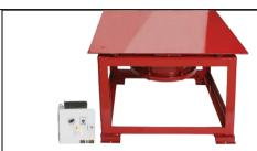
Table is 30" x 30" (762 x 762mm), and vibration is provided by an electromagnetic vibrator rated above 100lbs (45.5kg).
